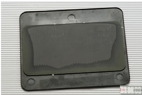
Fig. 17. Photograph of a half-cassette reoxidized at 600 °C and with a DoO of 10%; view of the substrate.
