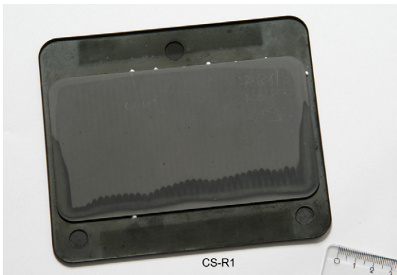
Fig. 16. Photograph of a half-cassette reoxidized at 600 °C to a DoO of 3%; view of the substrate.
