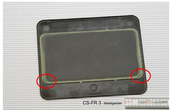
Fig. 18. Photograph of a half-cassette reoxidized at 800 °C to a DoO of 10%; view of the substrate, red ellipses highlight the macroscopic cracks.
